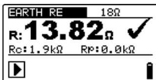
Figure 5.32: Example of earth resistance measurement result
