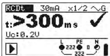
Figure 5.19: Example of trip-out time measurement results
