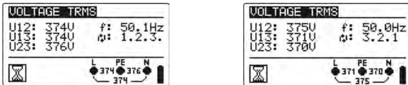
Figure 5.4: Examples of voltage measurement in three-phase system
