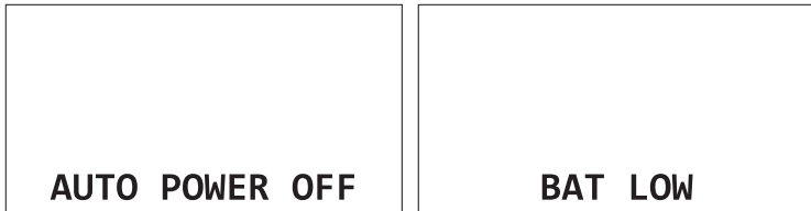
Fig. 5: Automatic power off Magnetometer is not operated for 20 minutes (left) The remaining battery capacity is too low (right)
