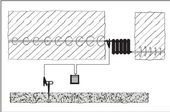
Fig. 4: Direct galvanic connection with earthing spike
