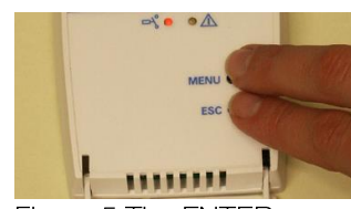
Figure 5 The ENTER command is done by pushing buttons MENU and ESC at the same time for about 14s.
