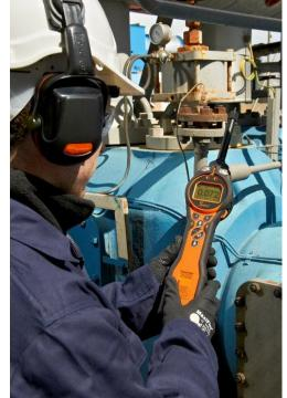
value of actual benzene present. Benzene concentrations are displayed down to ppb levels, giving you the most accurate, reliable data you can count on. Its unique IonPIDTM VOC sensor incorporates both Anti-contamination and Fence Electrode technology for extended operation in difficult working environments. Tiger Select is capable of providing 15-minute STELs and eight-hour TWAs for TACs.
