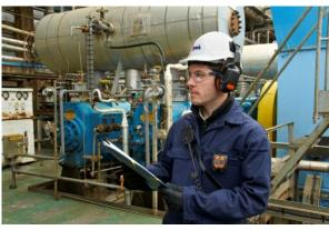
Cub<sup>TAC</sup> used to detect benzene at refinery.
