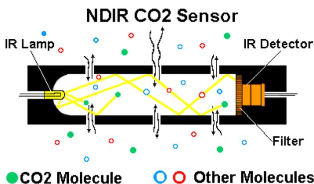
As shown in the figure, gas molecules diffuse into the sensing chamber. The IR light is directed through the sensing chamber towards the detector. The detector has a filter in front of it which eliminates all light except the 4.26 μm wavelength that CO<sub>2</sub> molecules can absorb. Since other gas molecules do not absorb light at this wavelength, only the CO<sub>2</sub> molecules affect the amount of light reaching the detector.
