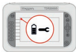
Current operational state. Currently in Setup operation
