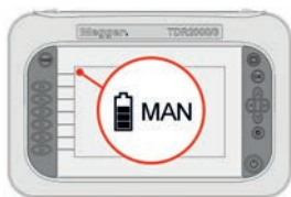
Current operational state. Currently in Manual operation
