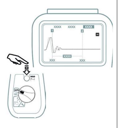
Hold key. When the rotary switch is set to cursor 1, cursor 2, or Auto, pressing the hold key will place an image of the current trace in grey on the display. This allows comparisons to be made between two cables or intermittent faults to be seen
