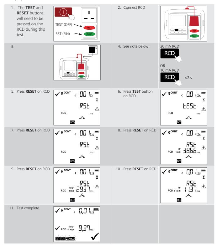
**NOTE:** The PAT250SX defaults to 30 mA RCD. To change to 10 mA, hold the RCD button down for more than 2 seconds then release.
