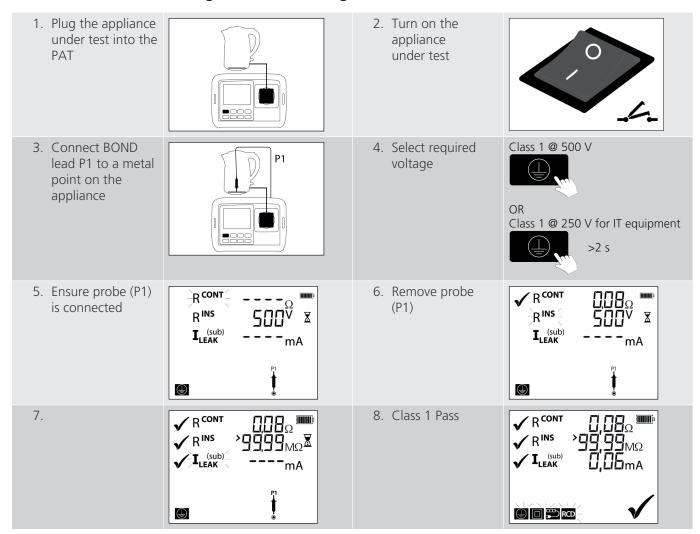
**NOTE**: If the contact symbol is displayed during the test, the PAT has detected an open circuit load. Ensure the appliance is switched on then press the Class 1 icon
