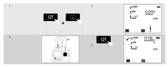
Example 2 – Class 2 250 V Insulation test
