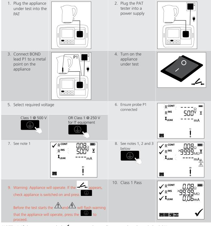
**NOTE**: 1: If the contact symbol \_\_\_ appears, the appliance needs to be switched ON.
