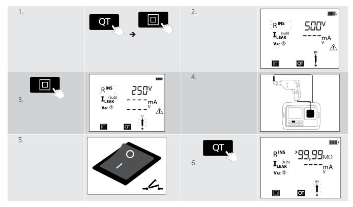
**Example 3** – Class 2 touch leakage test using the Substitute (or alternative) method.
