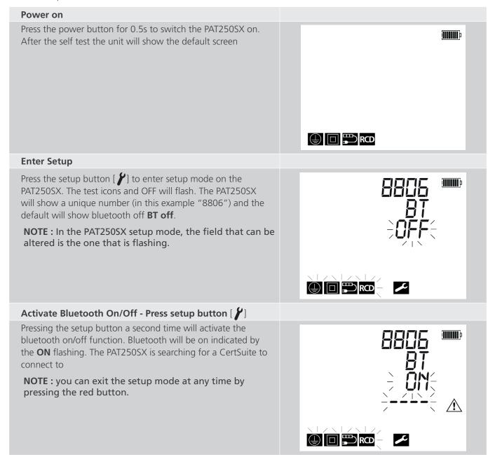
While **OFF** is flashing it can be changed. Press the setup button to change this to **ON**. The display will change to indicate Bluetooth is on **BT on**.
