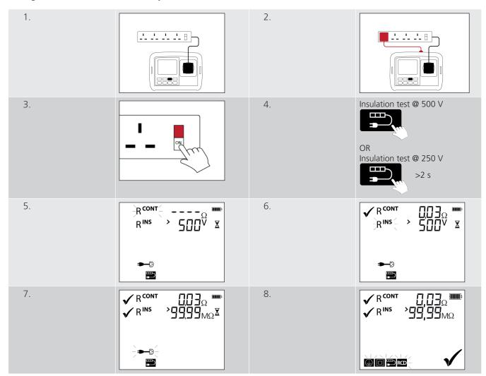
**NOTE:** Multiple earth continuity tests can be carried out by pressing the QT button during the continuity test, and pressing it again for each new continuity test. See 6.2 To repeat a continuity test (Class 1 and Extension lead tests only RCONT OR RPEO ) on page 17.
