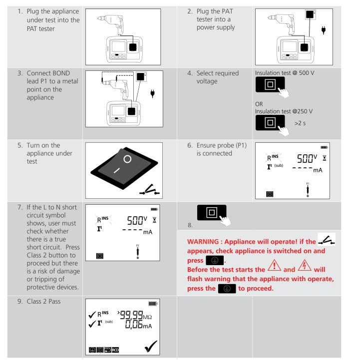
NOTE: High touch leakage measurement on faulty equipment can trip the supply RCD
