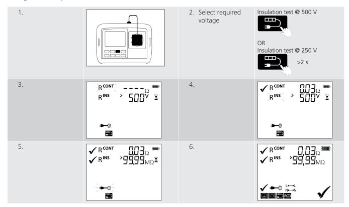
**NOTE**: For power cords longer than 5m the test can be re-run with a 1.0  $\Omega$  pass limit by pressing the test button within 5 seconds of the continuity test failing.
