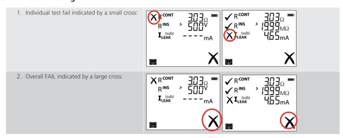
**NOTE**: Once an appliance has failed a test, further testing of the test group sequence is prevented for safety reasons, except for the extension lead testing
