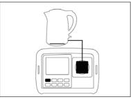
Connect the equipment to be tested to the instrument
