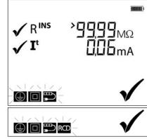
NOTE: High touch leakage measurement on faulty equipment can trip the supply RCD
