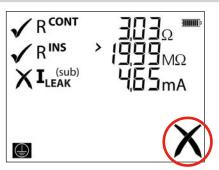
NOTE: Once an appliance has failed a test, further testing of the test group sequence is prevented for safety reasons, except for the extension lead testing
