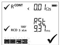
**Note**: The PAT150 defaults to 30 mA RCD. To change to 10 mA, hold the RCD button down for more than 2 seconds then release.
