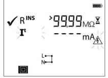
If the L to N short circuit symbol shows, user must check whether there is a true short circuit. Press Class II button to proceed but there is a risk of damage or tripping of protective devices.
