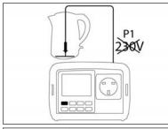
Connect the P1 test lead to socket P1 on the Pat100 and the probe to exposed metalwork Ensure the probe is NOT connected to a 230V source.
