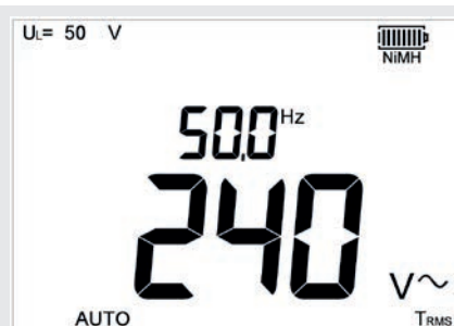
Figure 9: Instrument displaying that the circuit is live.
