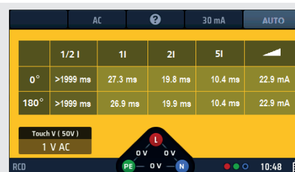
Fig 49: AUTO RCD test result progress
