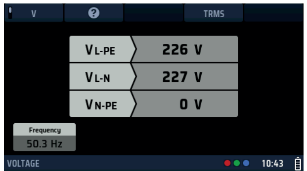
Fig 35: Voltage single phase
