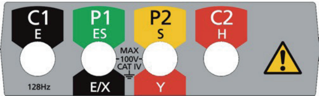
Test lead connections (at rear of instrument)
