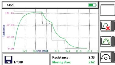
Use of the latest processors and a large internal memory allows for immediate calculations of resistivity (Wenner or Schlumberger method) and the ability to save a complete day's worth of test results.
