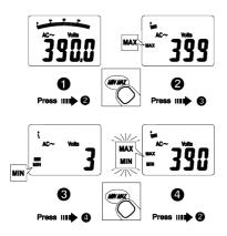
2: MAX: Meter is saving the maximum and minimum value. Maximum value is displayed
