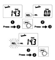
2: REL: Meter save the displayed offset value after one press of the ZERO button. The LCD is displaying the relative value.
