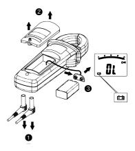
Low battery : "  $\boxdot$  " is displayed or flashes when a button pressed.
