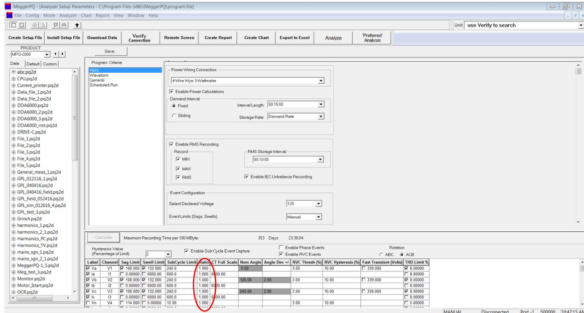
Figure 1: MeggerPQ software - Advanced Test Setup screen
