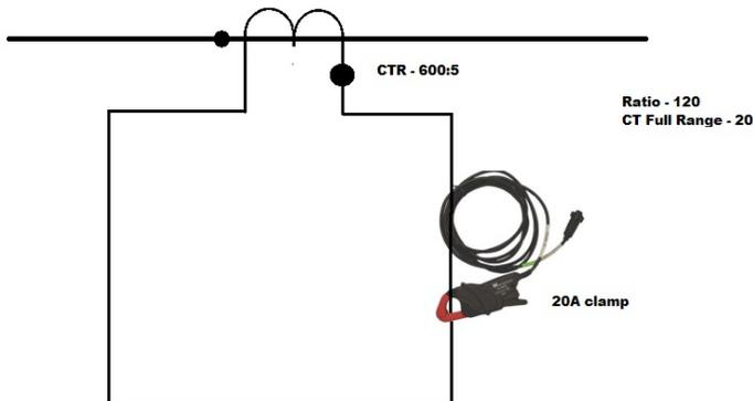
Figure 2: Connection diagram
