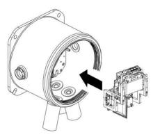
Hold the ribbon cable out of your way while you insert the Detection Module.
