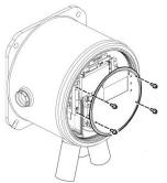
Use a 2mm allen-key to remove the four faceplate screws.
