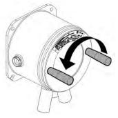
Turn counter-clockwise to unscrew the front cover.
