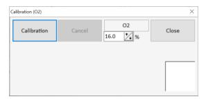
At this point click the calibration cap onto the sensor inlet port then open the valve on the manual fixed flow regulator. The screen on the ARA will then display C90 and begin counting down C89, C88 etc for approximately 20 seconds for the Oxygen ARA and 90 seconds for the other versions.
