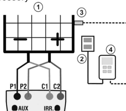
Fig. 15: Instrument's connection for IVCK tests with measurement of Irrad/Temp through SOLAR-02
