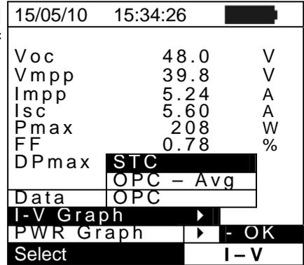
4. The graph is the I-V curve relative to the object under test translated to the standard conditions (STC) and referred to 1 module.
