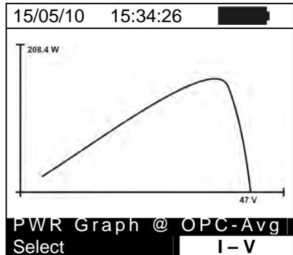
9. With screen of numerical values measured by the meter select the item “**PWR Graph**” by means of arrow key ▼ and press **ENTER** or the arrow key ►.
