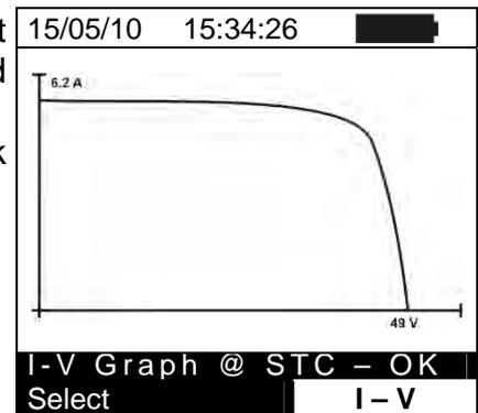
6. With screen of numerical values measured by meter select the item “**I-V Graph**” by means of arrow key ▼ and press **ENTER** or the arrow key ►.
