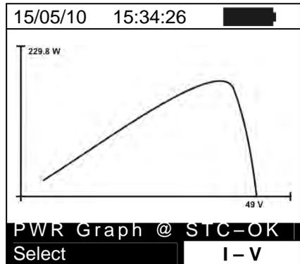
6. With screen of numerical values measured by meter, select the item “**PWR Graph**” by means of arrow key ▼ and press **ENTER** or the arrow key ►.
