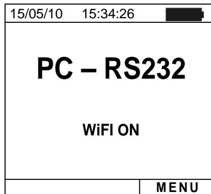
5. Enable the WiFi connection on the PC (if necessary, it is possible to use a WiFi adaptor). Select and connect the WiFi network which the instrument makes available in “Network connection → Wireless networks” section
