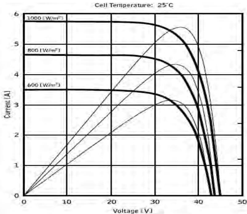
On each characteristic curve there is one single point in which the power transfer towards a hypothetical charge supplied by the photovoltaic module is maximized. The maximum power point corresponds to the voltage-current pair for which the product  $V \cdot I$  is maximum, where  $V$  is the value of voltage at the module's terminals and  $I$  is the current which runs in the circuit obtained by closing the module on a hypothetical charge.
