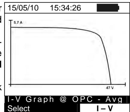
9. With screen of numerical values measured by meter select the item “**IV Graph**” by means of arrow key ▼ and press **ENTER** or the arrow key ►.
