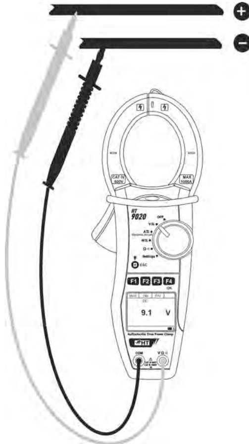
Fig. 5: DC Voltage measurement
