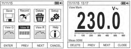
Fig. 19: Recalling measured data (snapshots) on the display
