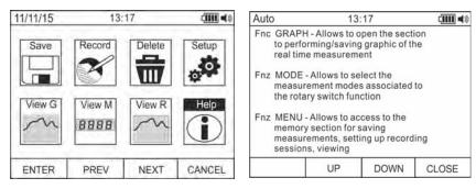
Fig. 21: Help on line on the display
