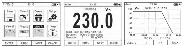
Fig. 20: Recalling recordings to the display
