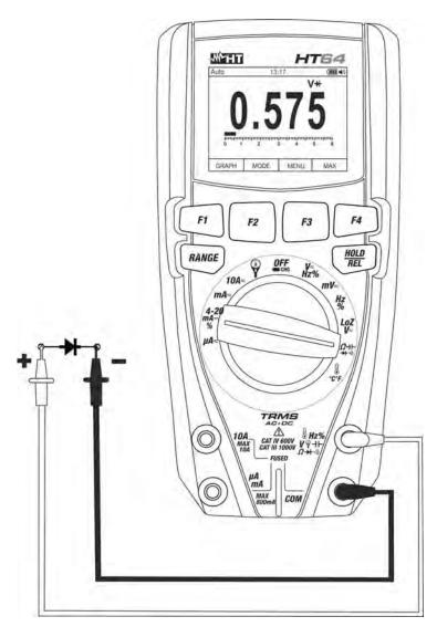
Fig. 27: Use of the instrument for diode test
