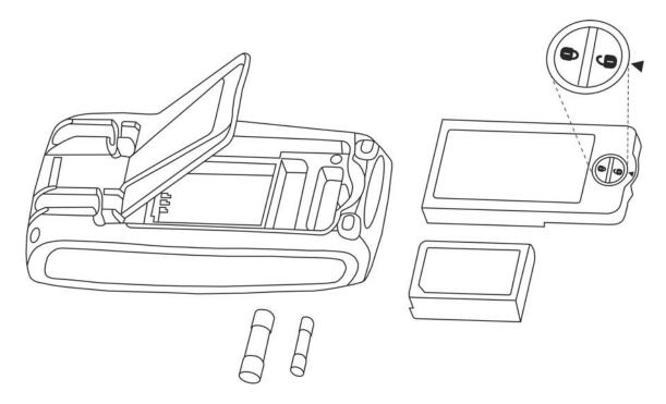
Fig. 34: Replacement of internal fuses
