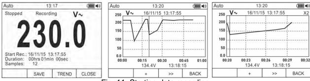
Fig. 11: Starting data recording
