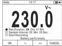
Fig. 10: Setting data recording
