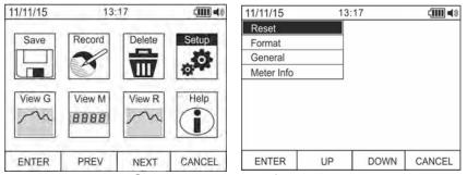
Fig. 13: General settings of the instrument
