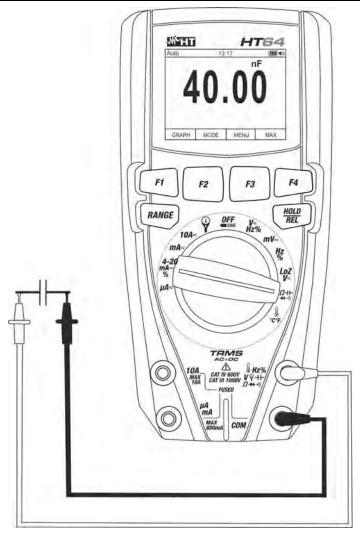
Fig. 28: Use of the instrument for Capacitance measurement
