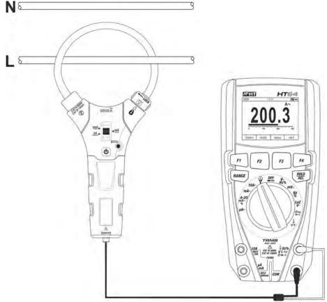
Fig. 32: Use of the instrument for DC/AC current measure with use of transducer clamp
