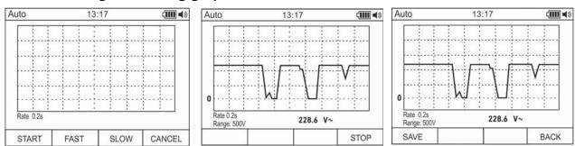
Fig. 8: Creating and saving a graph of measurements
