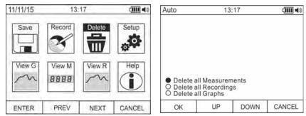
Fig. 12: Deleting the internal memory
