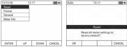
Fig. 14: Activating the instrument's reset
