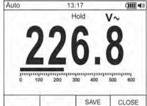
Fig. 4: Saving the value frozen on the display
