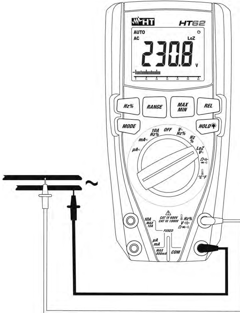
Fig. 4: Use of the instrument for AC/DC voltage measurement with low impedance (LoZ)
