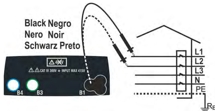
Fig. 35: Phase sequence check with test leads
