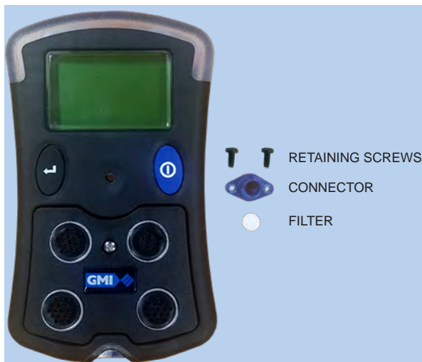
Fig. 4.4 Filter and Connector Removed
