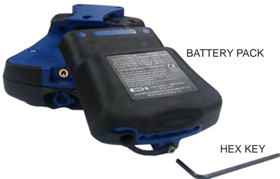
Fig. 4.11 Battery Pack Removed
