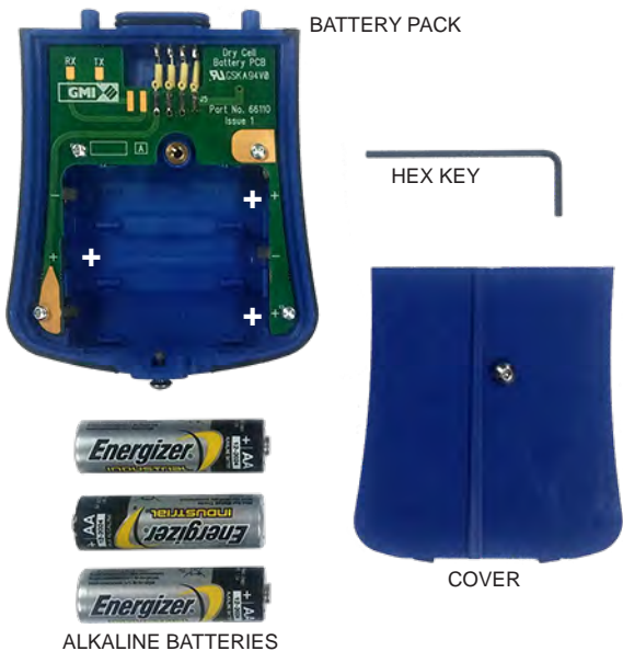
Fig. 4.13 Alkaline Batteries Removed
