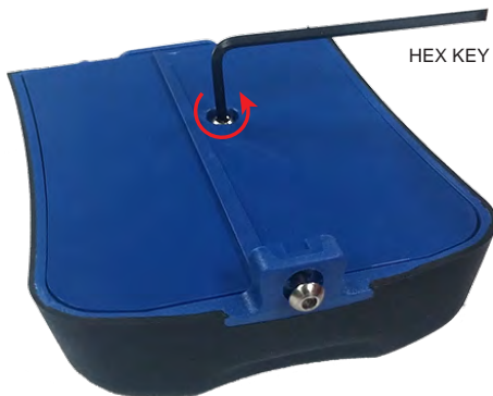
Fig. 4.12 Cover Plate Retaining Screw
