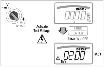
Auto-ranging is active during insulation resistance measurement.
