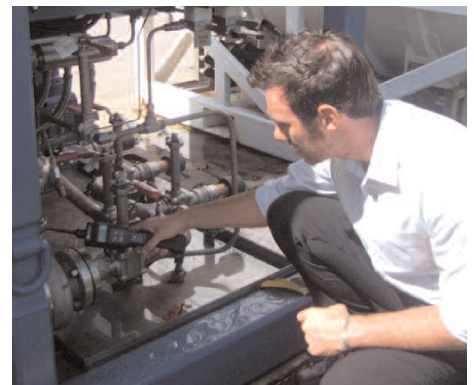
GasCheck 5000is being used to leak test machinery at PSL Energy Services, Singapore
