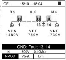
15.In case a fault is present (Rp<Lim) within the string, the instrument shows the screen to the side and the message (relevant to the example with NMOD = 14) "GND: Fault 8..9" on the display. Check the condition of the insulation of the junction boxes of the indicated modules and the relevant connection cables.</p>
