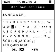
5. Use the arrow keys of the virtual keyboard to define a SAVE name for the module. Confirm with "**OK**""
