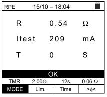
11.Press the **SAVE** key to store the test result in the instrument's memory (see § 7.1) or the **ESC/MENU** key to exit the screen without saving and go back to the main measuring screen.
