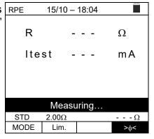
6. At the end of the compensation procedure, in case the measured resistance value is ≤5Ω, the instrument emits a double tone to signal the positive result of the test and displays the value of the compensated resistance of the cables, which will be subtracted from all the subsequent continuity measurements, at the bottom on the right side of the display.
