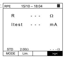
5. Press the **GO/STOP** key to start calibration. Messages "**Measuring...**" followed by "**Verification**" and "**Zeroing**" are shown in a sequence on the display.
