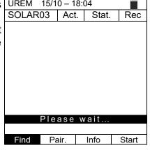
3. The instrument **activates the Bluetooth connection** and Solar shows the screen to the side for a few seconds, searching for a remote unit SOLAR03
