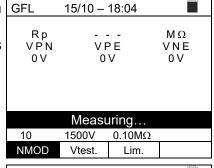
10. With no fault conditions (Rp≥Lim), the instrument shows the screen to the side and the message "OK" appears on the display.
