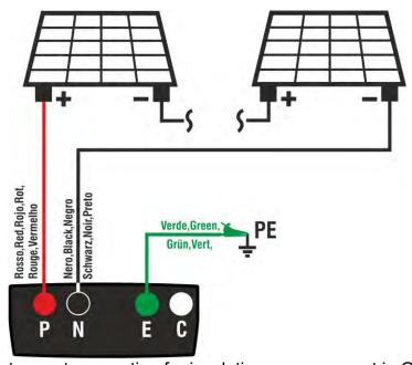
Fig. 9: Instrument connection for insulation measurement in GFL mode
