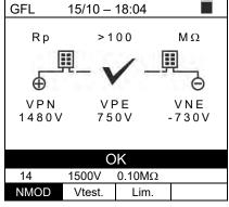
11. In case a fault is present (Rp<Lim) in position 0 (upstream of the first module), the instrument shows the screen to the side and the message "GND: Fault (+)..1" on the display. Check the condition of the insulation of the conductor (+) which comes from the string.
