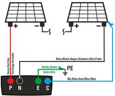
Fig. 10: Connection for IVCK tests without remote unit
