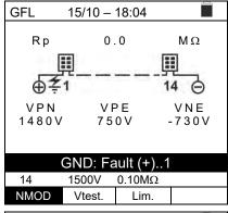
12. In case a fault is present (Rp<Lim) in position NMOD+1 (downstream of the last module), the instrument shows the screen to the side and the message "GND: Fault NMOD..(-)" on the display. Check the condition of the insulation of the conductor (-) which comes from the string.
