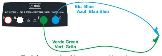
Fig. 5: Compensation of the measuring cables resistance
