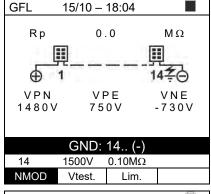
13. In case a fault is present (Rp<Lim) in position 1 (between module 1 and 2), the instrument shows the screen to the side and the message "GND: Fault 1..2" on the display. Check the condition of the insulation of the junction boxes of the indicated modules (1 and 2, in the example) and the relevant connection cables.
