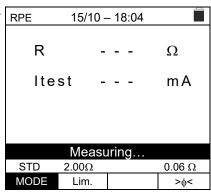
7. At the end of measurement, the instrument provides the value of resistance of the object being tested. If the result is lower than the set maximum limit value, the instrument shows the message "OK" (value lower or equal to the set limit threshold), otherwise it displays the message "NO OK" (value higher than the set limit threshold) as shown in the screen to the side.
