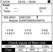
11. In case measurements are carried out without remote unit (see § 6.7.2), but the instrument has previously been paired to a remote unit, the message to the side appears on the display. Enter the remote unit's configuration menu (see § 6.2) and select "Unpair" to unpair the remote unit.
