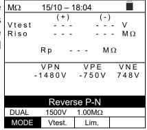
3. In DUAL mode, in case the instrument, upon pressing the GO/STOP key, detects a voltage VPN<15V, it stops measuring, gives out a long sound and the message "VPN<15VDC" appears on the display. Check the output voltage from the PV string, which must be ≥30V.
