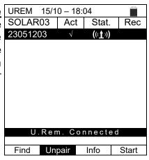
6. To start recording on an active and connected remote unit, use the arrow keys ◀ or ▶ and select "Start". The symbol "oo" will subsequently appear.
