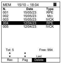
3. Press the **ENTER** key to confirm and the **ESC** key to exit without confirming and to go back to the main menu. **The** instrument always deletes the last saved measure
