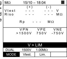
2. <u>In DUAL mode</u>, in case the instrument, upon pressing the **GO/STOP** key, detects a voltage **VPN** <**0V**, it stops measuring, gives out a long sound and the message **Reverse P-N**" appears on the display. Check polarity and the instrument's connections to the PV string.
