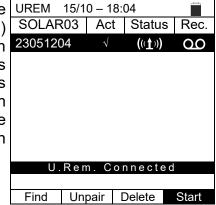
9. Bring the remote unit near the modules and connect the irradiance/temperature probes as shown in Fig. 11. Since recording has already been activated on remote unit SOLAR03, it is not strictly necessary to maintain the Bluetooth connection anymore. Maintaining the connection will only allow to immediately obtain the outcome of the test without waiting for the measuring campaign to be completed.
