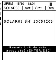
5. Confirm with ENTER on the instrument and on the remote unit SOLAR03 for pairing. From now on, the instrument and the remote unit are paired and it will not be necessary to repeat these operations. To connect the instrument to the remote unit, it will be sufficient to switch them on, bring them near to each other and wait for pairing.
