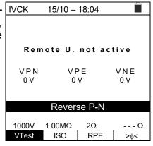
3. In case the instrument detects a voltage - 0.5V≤VPN≤15VDC at terminals P-N, it does not carry out the test, gives out a long sound and displays the message "VInput < 15VDC".
