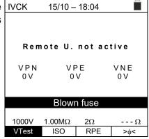
8. In case no recording has been activated on remote unit SOLAR03, the message to the side is shown on the display. Check the status of the remote unit SOLAR03
