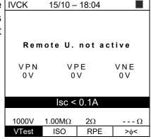
7. In case the instrument detects a blown fuse while measuring Isc current, the message to the side appears on the display. Please contact HT's After-sales Service.
