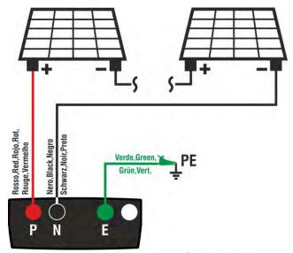
Fig. 4: Instrument connection for DMM Function
