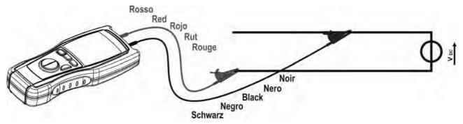
Fig. 2: Connection of the instrument's terminals during  $\ddot{V}$  test
