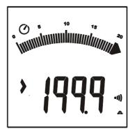
2. If the voltage present at the terminals is higher than 24V the instrument does not perform the test. The screen beside is displayed
