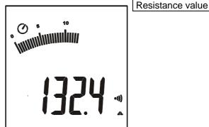
7. Example of display of resistance value. If such value is lower than  $2\Omega$  the instrument emits an acoustic signal
