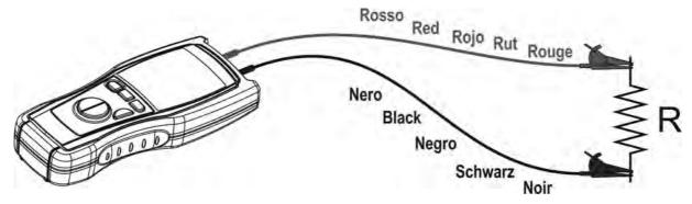
Fig. 4: Connection of the instrument's terminals during  $\Omega$ •••) test
