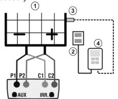
Fig. 15: Instrument's connection for IVCK tests with measurement of Irrad/Temp through SOLAR-02
