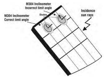
Fig. 8: Positioning the M304 inclinometer
