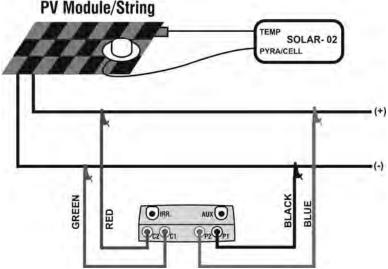
Fig.11: Connection of units to the PV module/string
