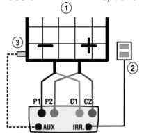
Fig. 14: Instrument's connection for IVCK tests with direct measurement of Irrad/Temp
