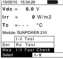
5. Press **ENTER**, select "**Settings**" and confirm by 15/05/10 pressing ENTER again to enter the following screen Module: where it is possible to set module type and number of modules making the string under test.
