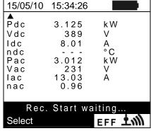
16. When the "00" instant after the press of **GO/STOP** key is reached, the recording starts and the units are correctly synchronized. In these conditions the message "**Rec running...**" is displayed on the main unit and the "**Recording...**" message is displayed on the SOLAR-02
