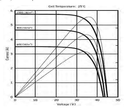
On each characteristic curve there is one single point in which the power transfer towards a hypothetical charge supplied by the photovoltaic module is maximized. The maximum power point corresponds to the voltage-current pair for which the product V\*I is maximum, where V is the value of voltage at the module's terminals and I is the current which runs in the circuit obtained by closing the module on a hypothetical charge.
