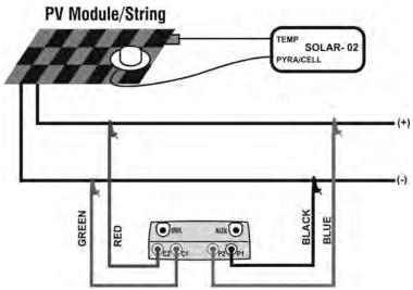
Fig. 9: Connection of units to the PV module/string
