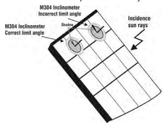
Fig. 10: Positioning the M304 inclinometer
