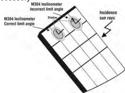
Fig. 7a: Instrument connection to module/string FV
