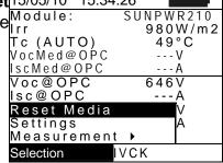
The average values are automatically reset even **modifying and saving** one of the following parameters:
