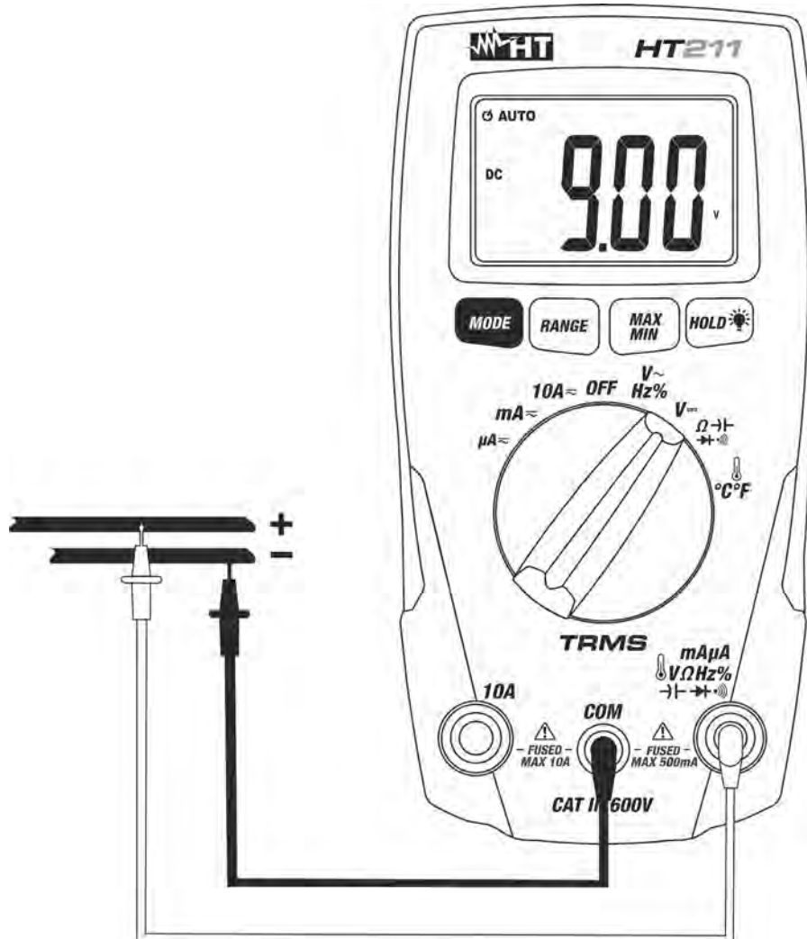
Fig. 2: Using the meter for DC Voltage measurement
