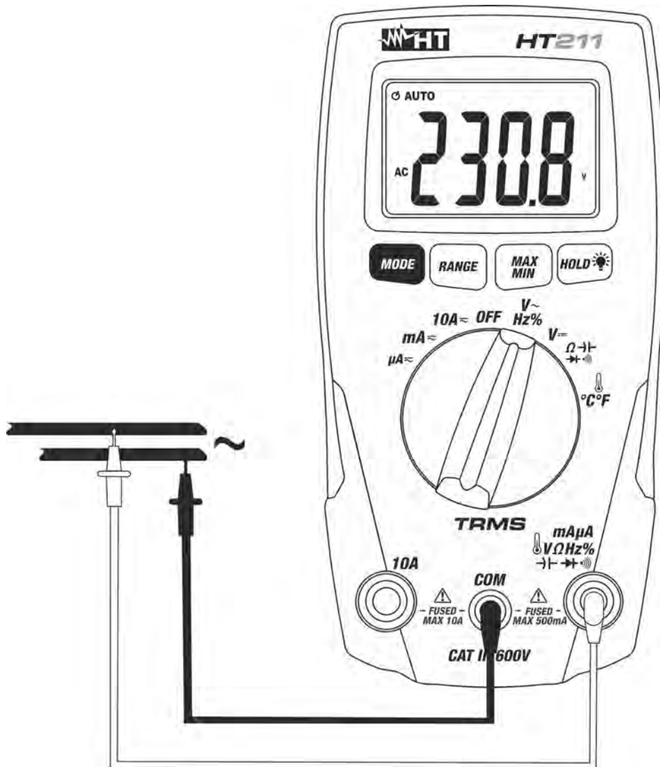
Fig. 3: Using the instrument for AC Voltage measurement
