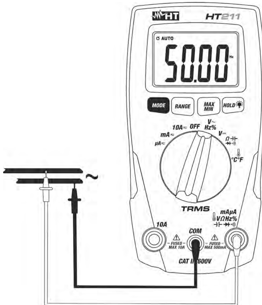
Fig. 4: Using the instrument for Frequency and Duty Cycle measurements
