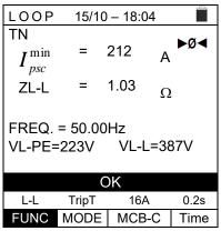
8. In case of **negative** result (minimum short-circuit current NOT interrupted by the protection device within the time indicated by the performed selections), the "**NOT OK**" message and the screen to the side are displayed by the instrument.  $I_{psc}^{min}$ ZL-L
