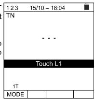
4. The instrument gives out a long sound until input voltage is present. At the end of phase L1 acquisition, the instrument is in standby, waiting for the signal on phase L2, and showing the "Disconnect L1" message, as shown in the screen to the side.
