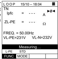
7. During this whole stage, do not disconnect the measuring leads of the instrument from the system under test. The following screen appears on the instrument's display.
