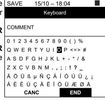
7. Press the SAVE/ENTER key to confirm saving the measure or ESC/MENU to exit without saving.
