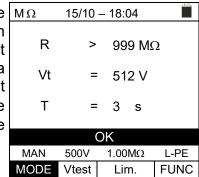
9. Press the **SAVE** key to store the test result in the instrument's memory (see § 7.1) or the **ESC/MENU** key to exit the screen without saving and go back to the main measuring screen.
