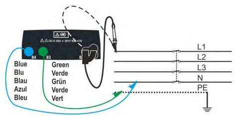
Fig. 7: Instrument connection by means of single cables and remote switch probe
