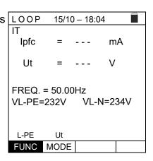
6. Press the **GO/STOP** key on the instrument, the **START** key on the remote switch probe or use the AutoStart feature (see § 5.1.5). The instrument starts the measurement and the "**Measuring...**" message is shown on the display. During this whole stage, do not disconnect the measuring leads of the instrument from the system under test. The following screen appears on the instrument's display.
