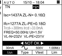
11. In case of a negative result of the Insulation test AUTO (insulation resistance < minimum limit threshold), the auto test is automatically blocked, the message "NOT OK" is shown and the screen to the side is displayed.
