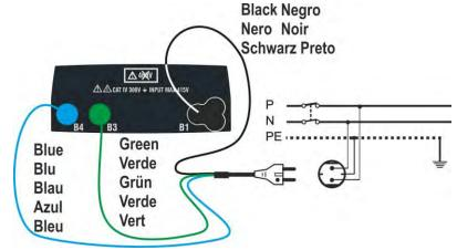
Fig. 6: Instrument connection through mains plug
