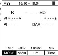
2. Press the GO/STOP key on the instrument or the START key on the remote switch probe. The instrument starts the measurement for the entire duration set, showing the "Measuring..." message. The instrument shows the message "OK" on the display in case of a positive result (value higher than the set minimum threshold) or "NOT OK" in case of a negative result (value lower than the minimum limit set).
