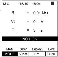
2. At the end of the test, if the measured resistance value is lower than the set limit, the instrument emits a long acoustic signal to indicate the negative result of the test and displays a screen like the one at the side.
