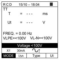
3. If the instrument detects a L-N or L-PE voltage higher than the maximum limit (265V), it does not carry out the test and displays a screen like the one to the side. Check the connection of measuring cables.
