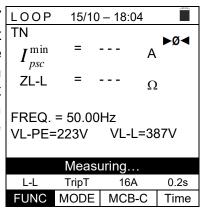
7. In case of **positive** result (minimum short-circuit current interrupted by the protection device within the time indicated by the performed selections), the "**OK**" message and the screen to the side are displayed by the instrument.  $I_{psc}^{min}$
