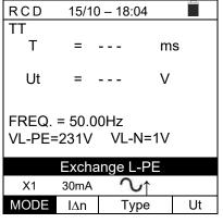
7. If the instrument detects the absence of the signal to terminal B3 (PE conductor), it provides the warning screen shown to the side and blocks the execution of the tests.
