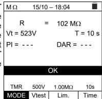
3. With a <u>measurement duration ≥ 60s</u>, the instrument MΩ shows the indication of the DAR parameter (Dielectric Absorbtion Ratio) as shown in the screen to the side.
