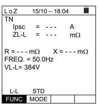
3. Press the GO/STOP key on the instrument to start the LoZ test. The following screen is shown on the display (in TN case of L-L measurement in STD mode). The standard (STD) prospective short-circuit current is shown on the display. The L-L Loop impedance values, in addition to its resistive and reactive components, are
