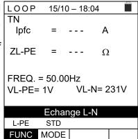
10. If the instrument detects that the phase and PE leads are inverted, it does not carry out the test and a screen similar to the one reported to the side is displayed. Check the connection of measuring cables.
