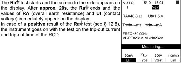
The **RCD** test starts and the screen to the side appears 7. on the display. The trip-out current and the trip-out time values appear on the display.
