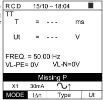
10. If the instrument detects a dangerous contact voltage Ut (above the set limit of 25V or 50V) in the initial pre-test, it provides the warning screen shown to the side and blocks the execution of the tests. Check the PE conductor and earth connection efficiency.
