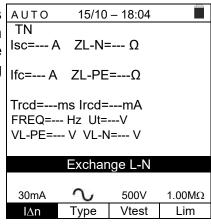
4. If the instrument detects a dangerous voltage on PE conductor, it does not carry out the test and displays a screen like the one to the side.
