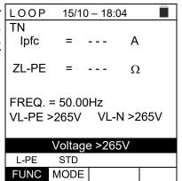
4. If the instrument detects a L-L voltage higher than the maximum limit (460V), it does not carry out the test and displays a screen like the one to the side. Check the connection of measuring cables.
