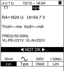
10. In case of a **negative** result of the **RCD test** (**Trcd** >300ms or **Ircd** > 33.0mA), the auto test is automatically blocked, the message "NOT OK" is shown and the screen to the side is displayed.
