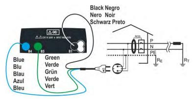
Fig. 17: Connection for single-phase 230V system by means of mains plug
