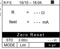
4. When using the  $> \phi <$  mode, in case the instrument detects a resistance higher than  $5\Omega$  at its terminals, it emits a prolonged acoustic signal, resets the compensated value and displays a screen like the one to the side.
