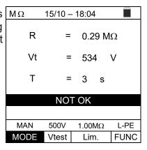
3. In AUTO mode, if the insulation measurement L-N is  $<50 k\Omega = 0.05 M\Omega$ , all the tests are completed or if the STOP key has been pressed, if RL-PE and RN-PE> Lim and Vt> Vnom, the instrument shows a screen like the one at the side. Disconnect the loads and resume the test.
