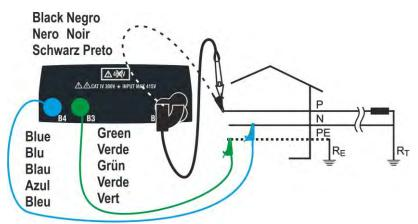
Fig. 24: P-N/P-PE test for single-phase/two-phase systems with cables and remote probe
