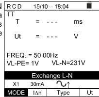
6. If the instrument detects that the phase and PE leads are inverted, it does not carry out the test and a screen similar to the one reported to the side is displayed. Check the connection of measuring cables.
