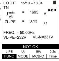
17. Press the **SAVE** key to store the test result in the instrument's memory (see § 7.1) or the **ESC/MENU** key to exit the screen without saving and go back to the main measuring screen.
