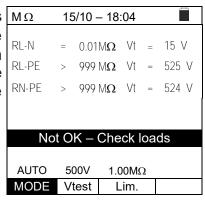
4. At the end of the test, if the value of the test voltage is lower than the nominal value, the instrument displays a screen like the one at the side.
