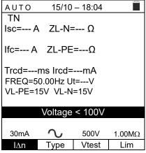
3. If the instrument detects that the phase and neutral leads are inverted, it does not carry out the test and a screen similar to the one reported to the side is displayed. Rotate the mains plug or check the connection of the measuring cables.
