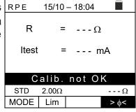
5. If the instrument detects a voltage higher than 3V at its terminals, it does not perform the test, emits a prolonged acoustic signal and displays a screen like the one to the side.
