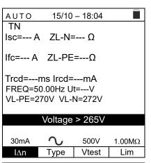
2. If the instrument detects a L-N or L-PE voltage lower than the minimum limit (100V), it does not carry out the test and displays a screen like the one to the side. Check that the system being tested is supplied.
