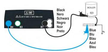
Fig. 8: Continuity test by means of single cables
