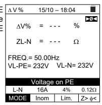
6. If the instrument detects the absence of the signal to terminal B1 (phase conductor), it provides the warning screen shown to the side and blocks the execution of the tests.
