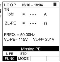
8. If the instrument detects the absence of the signal to terminal B1 (phase conductor), it provides the warning screen shown to the side and blocks the execution of the tests
