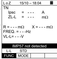
2. Connect the IMP57 to the instrument via the cable C2001 LoZ and to the powered system via the input terminals C1, C2 TN and P1, P2 placed on it (see the IMP57 user manual). The following screen appears on the display
