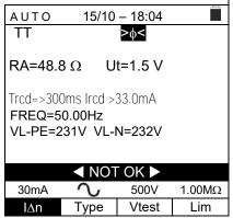
11. In case of a **negative** result of the **Insulation test** (insulation resistance < minimum limit threshold), the auto test is automatically blocked, the message "NOT OK" is shown and the screen to the side is displayed.
