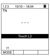
6. The instrument gives out a long sound until input voltage is present. At the end of the test, if the detected phase sequence is correct, the instrument displays a screen like the one shown to the side (result "123") and the "OK" message.
