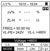
4. If the instrument detects a L-N or L-PE voltage higher than the maximum limit (265V), it does not carry out the test and displays a screen like the one to the side. Check the connection of measuring cables.
