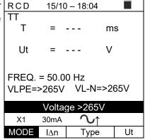
4. If the instrument detects a dangerous voltage on PE conductor, it provides the warning screen shown to the side and blocks the execution of the tests. Check the PE conductor and earth connection efficiency.
