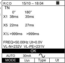
8. Press the **SAVE** key to store the test result in the instrument's memory (see § 7.1) or the ESC/MENU key to exit the screen without saving and go back to the main measuring screen.
