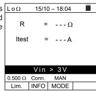
2. If the instrument does not detect the EQUITEST LoΩ accessory, it displays a screen like the one to the side. Check the connections with the accessory.
