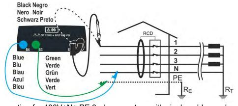
Fig. 19: Connection for 400V+N+ PE 3-phase system with single cables and remote probe
