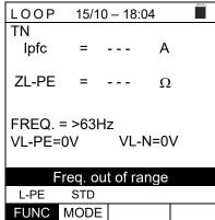
2. If the instrument detects a L-N or L-PE voltage lower than the minimum limit (100V), it does not carry out the test and displays a screen like the one to the side. Check that the system being tested is supplied.
