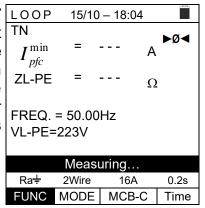
7. In case of **positive** result ( $Z_{L-PE} \le to$  limit impedance relative to protection device within the specified time – see § 12.10), the "OK" message and the screen to the side are displayed by the instrument.
