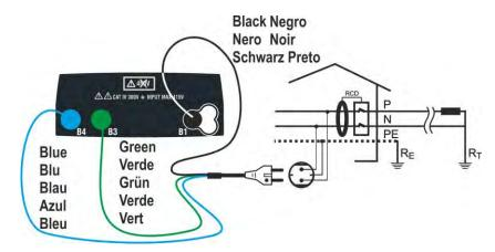
Fig. 4: Instrument connection through mains plug
