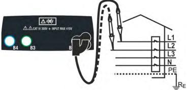
Fig. 33: Phase sequence check with remote switch probe
