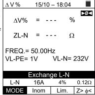
If the instrument detects that the phase and PE leads are inverted, it does not carry out the test and a screen similar to the one reported to the side is displayed. Check the connection of measuring cables.
