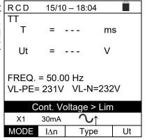
11. If the RCD does not trip within the maximum duration of the test, the instrument gives a long acoustic signal which signals the negative result of the test and then displays a screen similar to the one reported here to the side. Check that the set type of RCD matches the type of RCD being tested.
