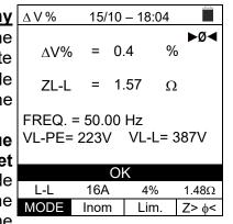
9. In case of negative result (maximum percentage value of calculated voltage drop according to § 12.11 > set limit value), the "NOT OK" outcome and the screen to the side are displayed by the instrument. The screen contains the value of the Z2 end-of-line impedance together with the Z1 (Offset) value.
