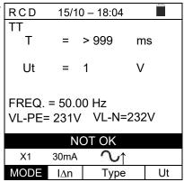
12. If the instrument detects, at the input terminals, too high an external impedance so that it cannot let the nominal current flow, it provides the warning screen shown to the side and blocks the test. Disconnect the possible loads downstream of the RCD before performing the test
