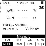
7. If the instrument detects the absence of the signal to terminal B4 (neutral conductor), it provides the warning screen shown to the side and blocks the execution of the tests.  $\Delta V \%$
