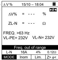
2. If the instrument detects a L-N or L-PE voltage lower than the minimum limit (100V), it does not carry out the test and displays a screen like the one to the side. Check that the system being tested is supplied.
