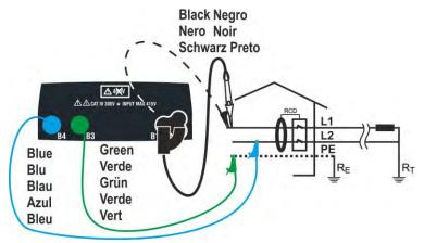
Fig. 20: Connection for L-L-PE 2-phase system with single cables and remote probe
