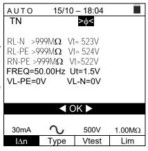
9. In case of a **negative** result of the Rattest (Z<sub>L-N</sub> and/or AUTO  $Z_{L-PE} > 199\Omega$ ), the auto test is automatically blocked, the message "NOT OK" is shown and the screen to the side is displayed.
