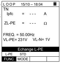
11. If the instrument detects a dangerous contact voltage Ut (above the set limit of 25V or 50V) in the starting pre-test, it provides the warning screen shown to the side and blocks the execution of the tests. Check the PE conductor and earth connection efficiency.
