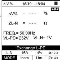
11. If the instrument detects a VL-PE, VL-N or VN-PE >5V during the test leads' calibration, it does not carry out the test and a screen similar to the one reported to the side is displayed. Check the connection of measuring cables.
