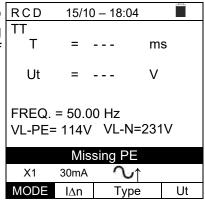
8. If the instrument detects the absence of the signal to terminal B4 (neutral conductor), it provides the warning screen shown to the side and blocks the execution of the tests.
