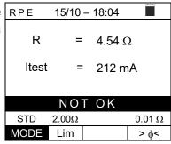
2. If the instrument detects a resistance higher than the full RPE scale, it emits a prolonged acoustic signal and displays a screen like the one to the side.
