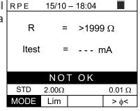
3. When using the >φ< mode, in case the instrument detects a calibration reset (performing the operation with open terminals), the instrument gives out a long sound and displays a screen like the one to the side.
