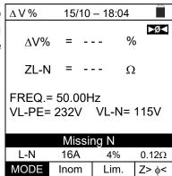
8. If the instrument detects the absence of the signal to terminal B3 (PE conductor), it provides the warning screen shown to the side and blocks the execution of the tests.
