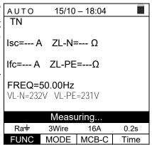
7. In case of positive result (Z<sub>L-PE</sub> ≤ to limit impedance relative to protection device within the specified time – see § 12.10), the "OK" message and the screen to the side are displayed by the instrument.
