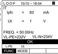
8. In case of **negative** result (contact voltage at the point >50V or >25V), the "**NOT OK**" message and the screen to the side are displayed by the instrument.
