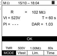
With a <u>measurement duration ≥ 600s</u>, the instrument shows the indication of the DAR parameter (Dielectric Absorbtion Ratio) and of the PI prameter (Polarisation Index) as shown in the screen to the side.
