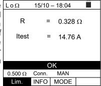
7. Press the **SAVE** key to store the test result in the instrument's memory (see § 7.1) or the **ESC/MENU** key to exit the screen without saving and go back to the main measuring screen.
