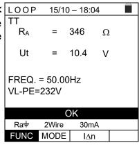
8. In case of **negative** result (**overall earth resistance** RA > LOOP (**Utlim/IΔn**), the "**NOT OK**" message and the screen to the side are displayed by the instrument. The screen contains the contact voltage value on the secondary display.
