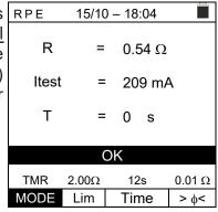
4. Press the **SAVE** key to store the test result in the instrument's memory (see § 7.1) or the **ESC/MENU** key to exit the screen without saving and go back to the main measuring screen.
