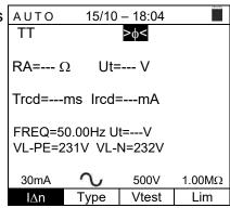
5. Press the **GO/STOP** key on the instrument or the **START** key on the remote switch probe. The instrument will start the automatic test sequence.
