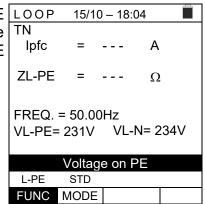
6. If the instrument detects the absence of the signal to terminal B4 (neutral conductor), it provides the warning screen shown to the side and blocks the execution of the tests.
