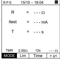
2. Press the **GO/STOP** key on the instrument or the **START** key on the remote switch probe. The instrument starts a series of continuous measurements for the entire duration set with a countdown, giving a short beep every 3 seconds and alternating the words "**Measuring...**" and "**Please wait...**".
