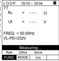
7. In case of **positive** result (**overall earth resistance** R<sub>A</sub> < LOOP (**Utlim/I**Δ**n**), the "**OK**" message and the screen to the side are displayed by the instrument. The screen contains the contact voltage value on the secondary display.
