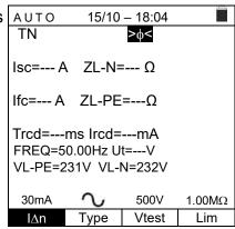
5. Press the **GO/STOP** key on the instrument or the **START** key on the remote switch probe. The instrument will start the automatic test sequence.
