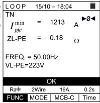
8. In case of **negative** result ( $Z_{L-PE}$  > **to limit impedance** relative to protection device within the specified time – see § 12.10), the "**NOT OK**" message and the screen to the side are displayed by the instrument.
