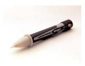
The non-contact volt stick can provide the electrical contractor with a simple means of checking whether a circuit is live or dead by holding the tip close to the phase conductor of the circuit under test.
