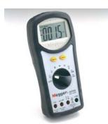
While most of these units are generally capable of indicating or even measuring voltages up to 1000 or 500 V a.c./d.c. they are not approved for confirming whether a circuit is live or dead because they do not have fixed test leads.
