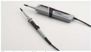
Electronic versions of the test lamp voltage tester are now very common and are generally divided into two variants. One has a LED ladder display that is divided into set voltages while the other has a LCD display that can display voltages in 1 volt increments. The ranges of these units are usually from 6 to 1000 V a.c. / d.c.
