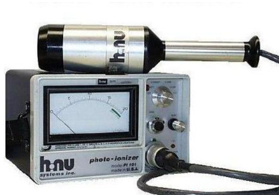
HNU PI101 – the first photoionisation detector, developed in 1974.
