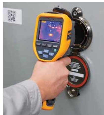
Combine with a Fluke ClirVu™ Infrared Window to conduct thermal inspections without having to open the electrical panel.
