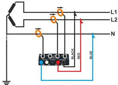
Fig. 15: Connection for measurement on Two-phase system 3-wires 36-Y Open
