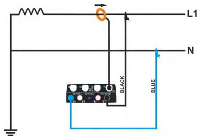
Fig. 9: Connection for measurement on single-phase 16-2WIRES
