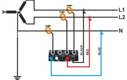
Fig. 16: Connection for measurement on Two-phase system 3-wires 36-2EI. 1/2
