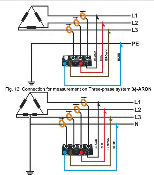
Fig. 13: Connection for measurement on Three-phase system 4-wires 36-High Leg
