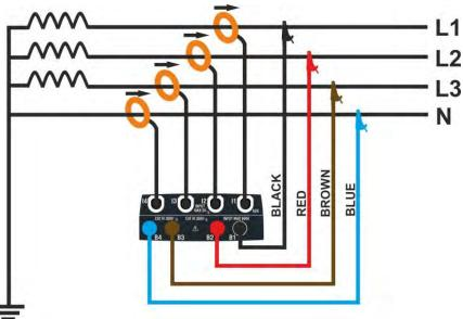
Fig. 10: Connection for measurement on Three-phase system 36-4WIRES
