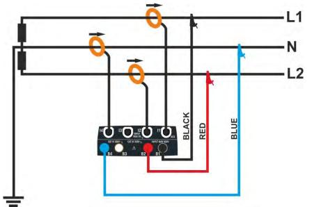
Fig. 17: Connection for measurement on Two-phase system 3-wires 16- CentrePoint
