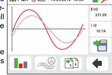
Press the **SAVE** button or touch the  $\square$  icon to save the measurement on the display as instantaneous snapshot (see § 7.1).
