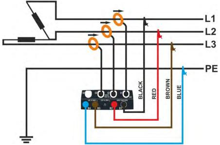
Fig. 14: Connection for measurement on Three-phase system 3-wires 3ϕ-∆ Open
