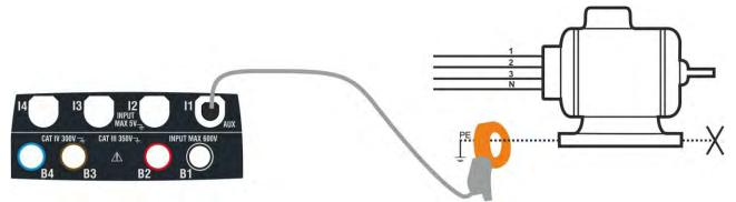
Fig. 7: Direct measurement of leakage current in three-phase systems
