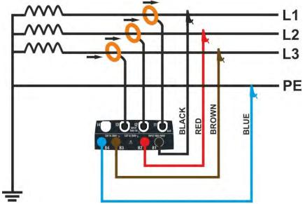
Fig. 11: Connection for measurement on Three-phase system 36-3WIRES
