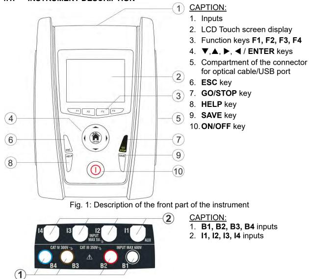
Fig. 2: Description of the upper part of the instrument
