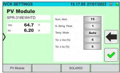
Fig. 55: I-V curve measurement parameter settings
