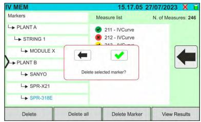
Fig. 81: Deleting an internal marker
