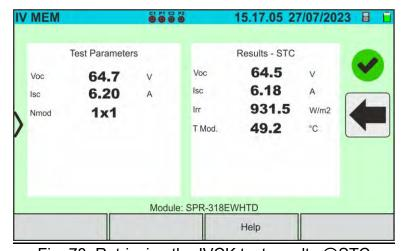
Fig. 78: Retrieving the IVCK test results @STC
