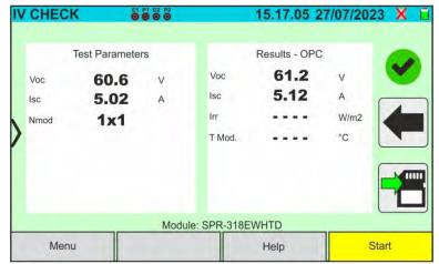
Fig. 50: Example of a positive IVCK test result - OPC values 12. If the result is **negative**, the following screen is shown:
