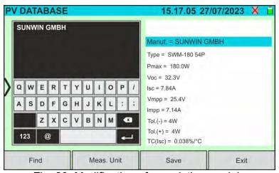
Fig. 28: Modification of an existing module
